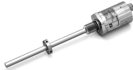
Figure 7 – Product: HYPERWAVE WRG-A magnetostrictive position transducer, 316 stainless steel stem, IP67 environmental protection, fixing by threaded flange
