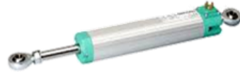
Figure 3 – Product: PCM potentiometric position transducer body in anodized aluminum IP65, fixing by self-aligning joints
