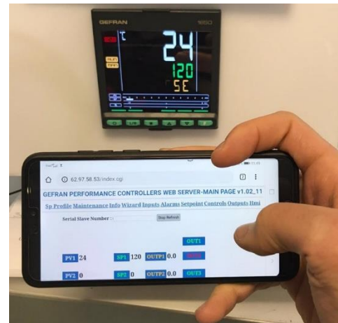
Figure 3 –Webserver remote connection
